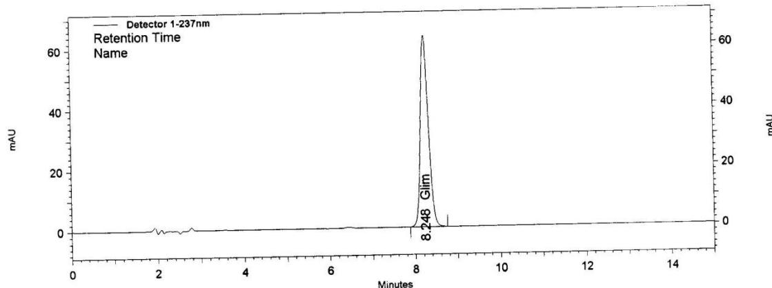
Figure 3.3: The chromatogram of a sample containing glimepiride under the chromatographic conditions.
